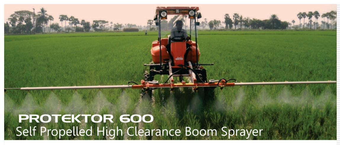
**SHAKTIMAN** PROTEKTOR is especially designed for wider range and coverage of crops to spray all types of pesticides, weedicides and fungicides. High ground clearance ensures no damage for tall ground crops like Cotton, Sunflower, Paddy, Chilli etc. Its compact design, hydrostatic and hydraulic system enable it to perform spraying operation easily and effectively.
