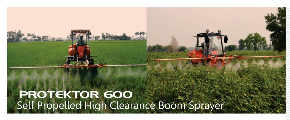
**SHAKTIMAN** PROTEKTOR is especially designed for wider range and coverage of crops to spray all types of pesticides, weedicides and fungicides. High ground clearance ensures no damage for tall ground crops like Cotton, Sunflower, Paddy, Chilli etc. Its compact design, hydrostatic and hydraulic system enable it to perform spraying operation easily and effectively.
